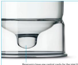
Reservoirs have one central cavity for the inlet filter to allow the most efficient delivery of mobile phase to HPLC analyzers
